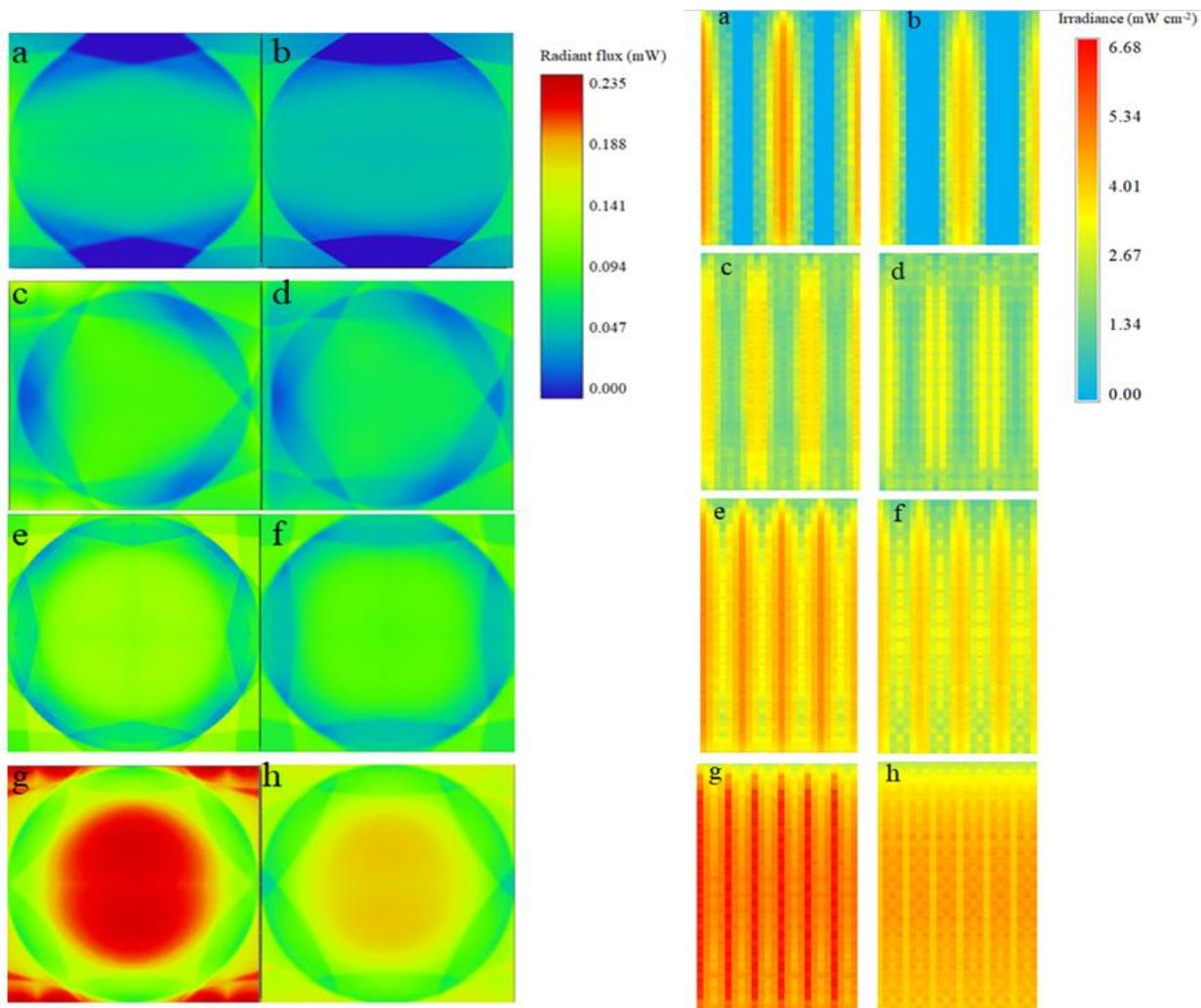
**Figure 2.** Light profiles obtained with Zemax OpticStudio software: a) 2 LED columns, 10 mm away; b) 2 LED columns, 15 mm away; c) 3 LED columns, 10 mm away; d) 3 LED columns, 15 mm away, e) 4 LED columns, 10 mm away; f) 4 LED columns, 15 mm away; g) 6 LED columns, 10 mm away; h) 6 LED columns, 15 mm away
