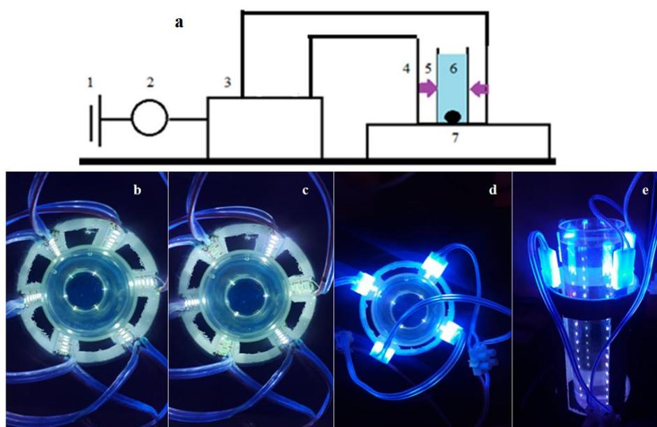
**Figure 1.** Experimental setup. (a) 1 - energy source, 2 - power meter, 3 - LED control board, 4 - LED columns, 5 - UV rays reaching the reactor, 6 – reactor, and 7 - magnetic stirrer. Below, upview of (b) arrays #LED = 6,  $D_w = 15$  mm; (c) #LED = 3,  $D_w = 15$  mm; and (d), #LED = 4,  $D_w = 10$  mm. Side view of #LED = 4,  $D_w = 10$  mm (e).
