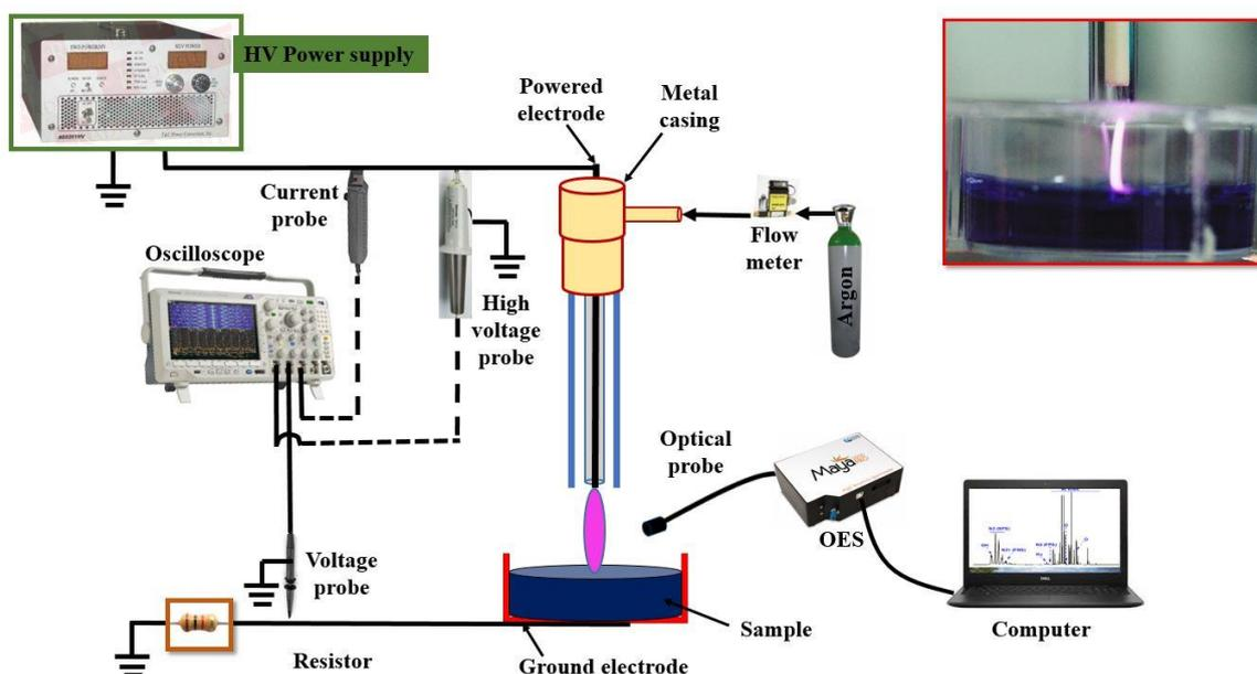
**Figure 1.** Schematic diagram (left) and picture (right) of the plasma jet over the liquid surface.
